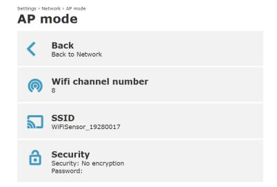
At the AP mode Wi-Fi sensor have own DHCP and DNS server. Network parameters are stated below (parameters are not configurable from web). When Wi-Fi sensor at AP mode is configured from cell phone, it is recommended to deactivate mobile data.
