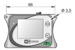
Device can be mounted onto wall by optional holder ATRU-AC02 –
