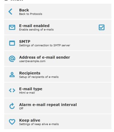
Proper settings of SMTP parameters can be tested at Advanced options menu accessible from main page. At first step need to be email and SMTP connection properly set at settings. After that email can be tested. Return codes are described at table below.
